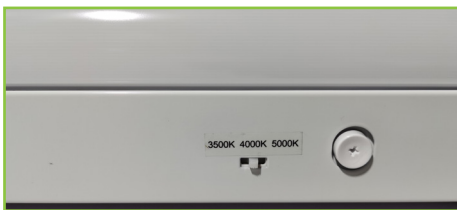
Field Adjustable CCT Switch (Factory Installed Standard for All Fixtures - This Allows Fixture CCT to Be Field Adjustable from 3500K, 4000K, 5000K)
