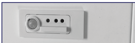
Integrated EasySense Sensor (-P2)
